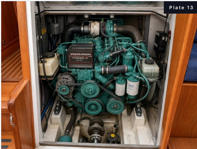
Plate 13. Volvo Penta TMD22-P in engine bay; clean, no active leaks.
