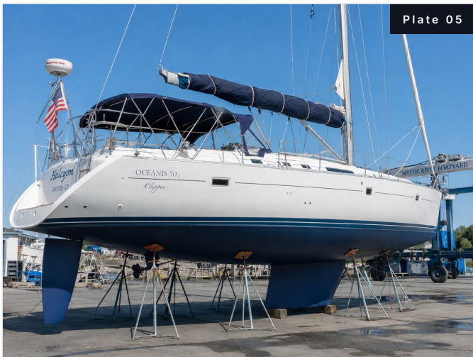
Plate 05. Port underbody after pressure-wash; fair, with serviceable antifouling.
