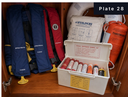
Plate 28. Stowed PFDs and distress kit; flares expired (A-1).
