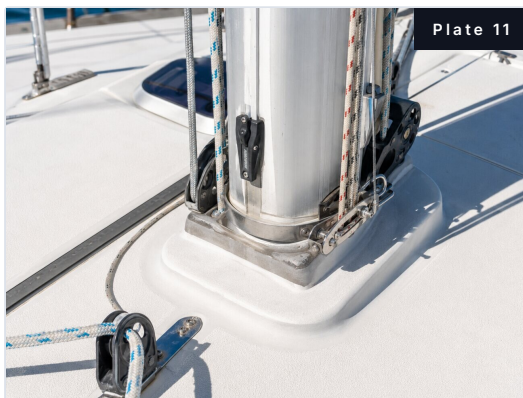
Plate 11. Mast base, collar, and deck partners; sound, no compression set.
