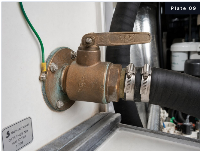
Plate 09. Representative bonded bronze seacock, engine bay; valve exercised, sound.
