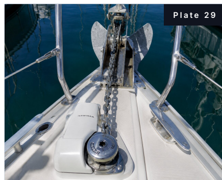
Plate 29. Electric windlass and primary anchor on the bow roller.
