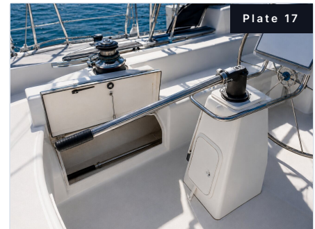
Plate 17. Emergency tiller stowed and test-fitted to the stock head.
