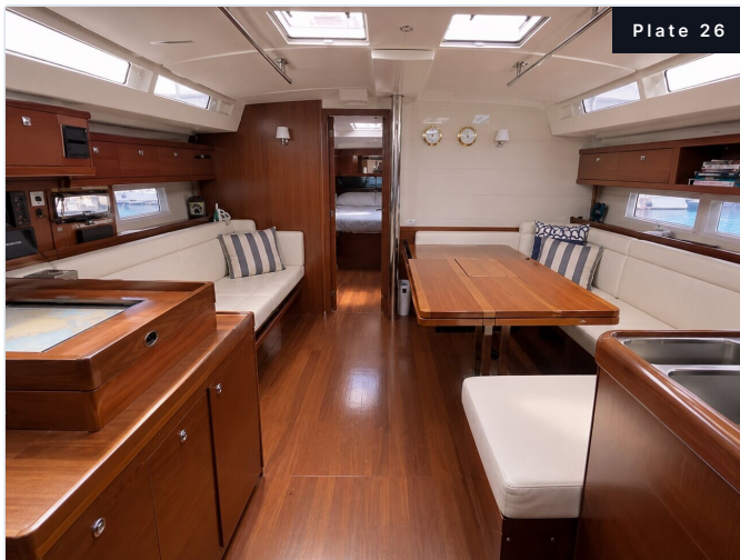
Plate 26. Main saloon and settees; joinery sound, no water staining.
