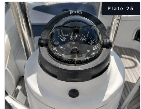
Plate 25. Pedestal-mounted steering compass; card free, lighting operable.
