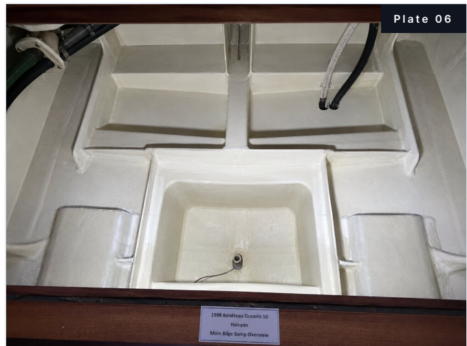
Plate 06. Moulded grid and main bilge sump, dry and clean; bonding intact.
